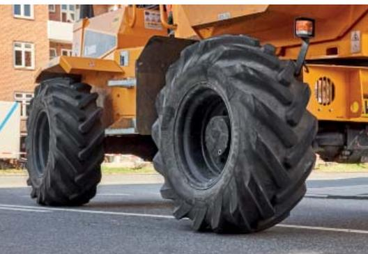
Our tyres are sufficiently flexible to endure the stresses of tight manoeuvring under heavy loads, without impairing the steering and handling characteristics of the machine. The overall design and construction of the carcass ensure excellent lateral stability. A fully loaded dumper fitted with STARCO Dumper tyres easily maintains lateral stability above the regulatory minimum tilt-test required in most European countries and outperforms all comparable competitors.
