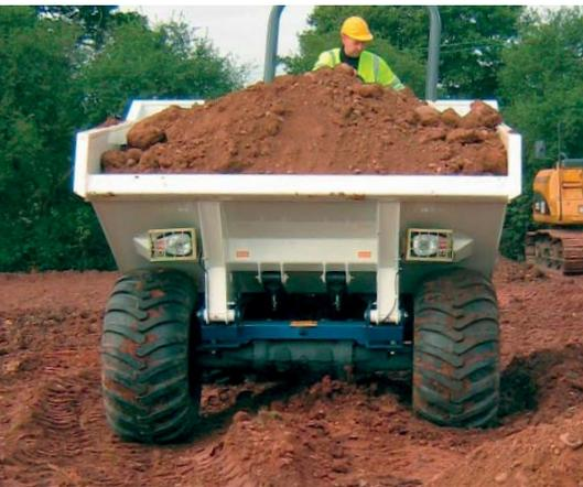
The STARCO Dumper tyre is of **bias belted design** - the preferred choice of the construction industry due to its **superior ability** to withstand sidewall impact and **excellent lateral stability** compared to radial tyres.
