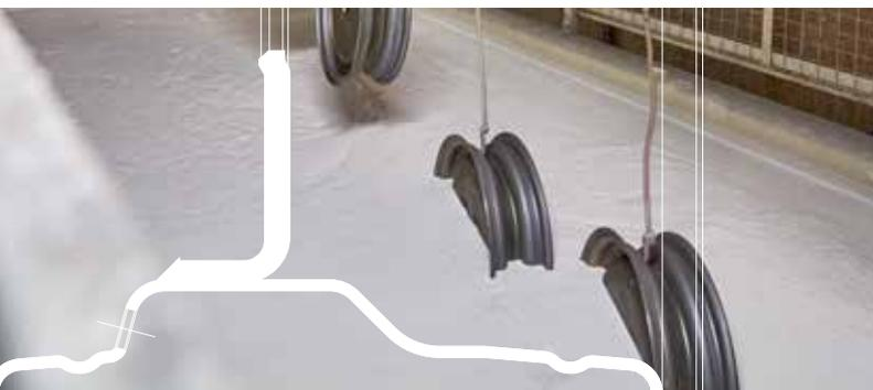
All steel wheels manufactured by STARCO are e-coated to prevent rust and corrosion and can be painted in any colour.
