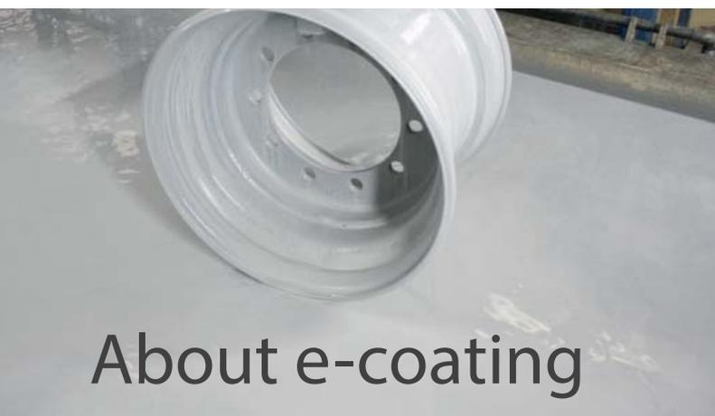
The e-coat is an electrodeposition coating process, in which steel wheels are given a priming coat that will prevent rust and corrosion throughout the normal working life of the wheel.
