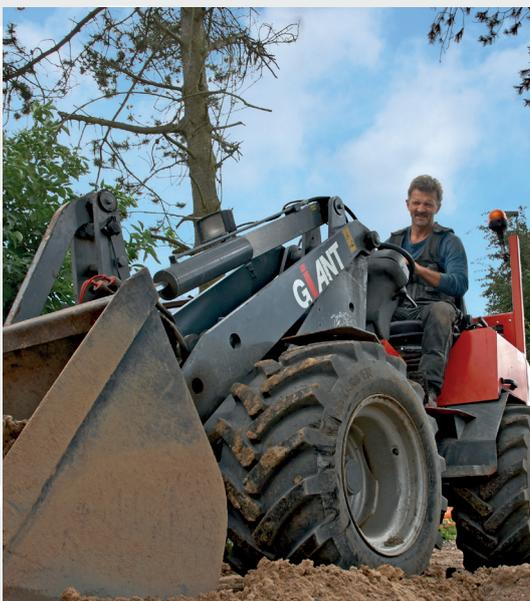
STARCO Dumper tires are of bias belted design - the preferred choice of the dumper industry due to its excellent lateral stability and superior capacity to withstand sidewall impact.
